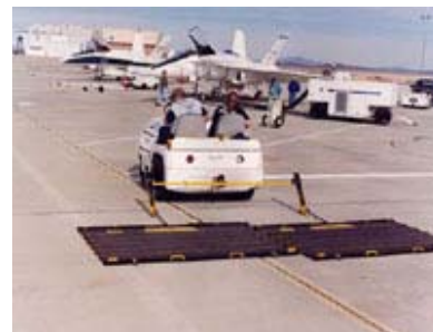
Kay and Associates employees Scott Rogers and Tim Coghlan use the FOD BOSS tools to sweep the flightline. NASA Photo / Tony Landis
